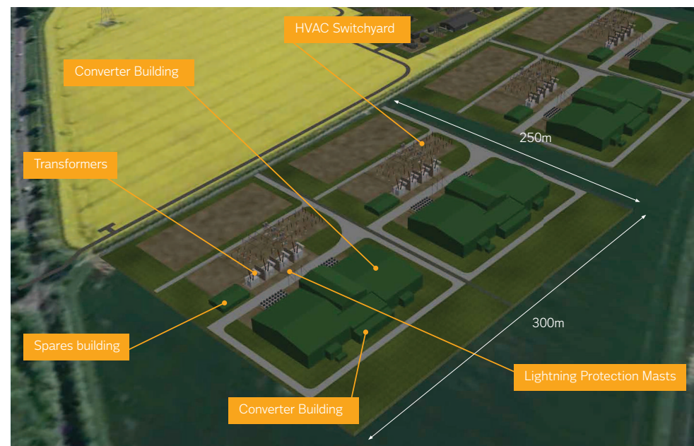
3D visualisation of project substation (HVDC option)
